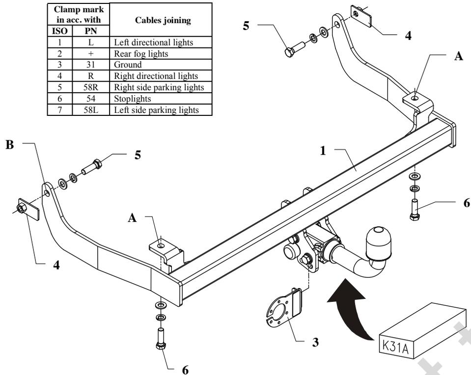
This towing hitch is designed to assembly in following cars: **VOLKSWAGEN CADDY, passenger car/delivery van**, produced since 11.1995 till 01.2004 and **SEAT INCA, passenger car/delivery van** produced since 11.1995 till 06.2003, catalogue no. **K31A** and is prepared to tow trailers max total weight **1100kg** and max vertical load **50 kg**.
