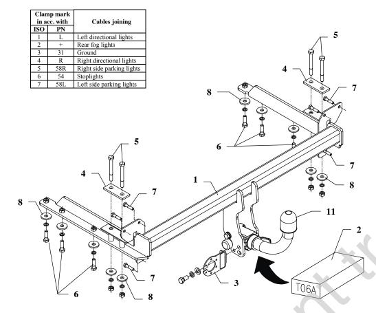
This towbar is designed to assembly in following cars: **KIA SEPHIA II, 4 doors, KIA SHUMA II, 5 doors (FB),** produced since 10.1997 till 12.2004, catalogue no. **T06A** and is prepared to tow trailers max total weight **1350 kg** and max vertical load **50 kg**.
