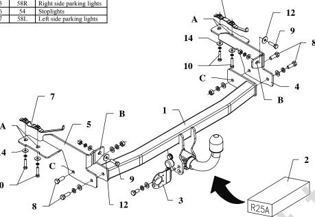
This towbar is designed to assembly in following cars: **FIAT PUNTO II, 3/5 doors VAN (188), except Sport,** produced since 09.1999 till 2011, catalogue no. **R25A** and is prepared to tow trailers max total weight **1400 kg** and max vertical mass **75 kg**.
