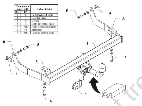
This towing hitch is designed to assembly in following cars: **VOLKSWAGEN CADDY**, passenger car/delivery van, produced since 11.1995 till 01.2004 and SEAT INCA, passenger car/delivery van produced since 11.1995 till 06.2003, catalogue no. K31A and is prepared to tow trailers max total weight 1100kg and max vertical load 50 kg.
