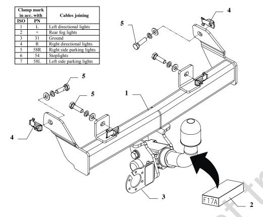
This towing hitch is designed to assembly in following cars: **PEUGEOT 106, 3/5 doors, (1A, 1C),** produced since 09.1991 till 04.1996, catalogue no. **F17A** and is prepared to tow trailers max total weight **1054** kg and max vertical load **50** kg.
