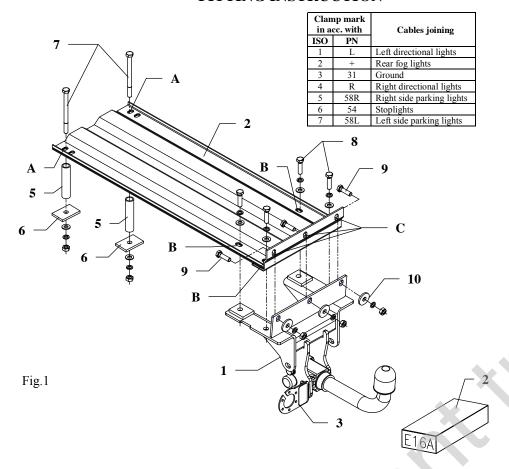
This towbar is designed to assembly in following car: **OPEL OMEGA** "B" 4 doors, produced since 04.1994 till 07.2003, catalogue no. **E16A** and is prepared to tow trailers max total weight **2100** kg and max vertical load **75** kg.
