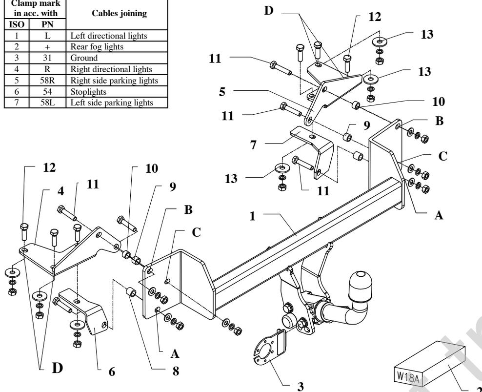
This towing hitch is designed to assembly in following car: **SUZUKI LIANA, 5 doors, ESTATE, 4WD**, produced since 05.2001 till 12.2007, catalogue number **W18A** and is prepared to tow trailers max total weight **1200 kg** and max vertical load **60 kg**.
