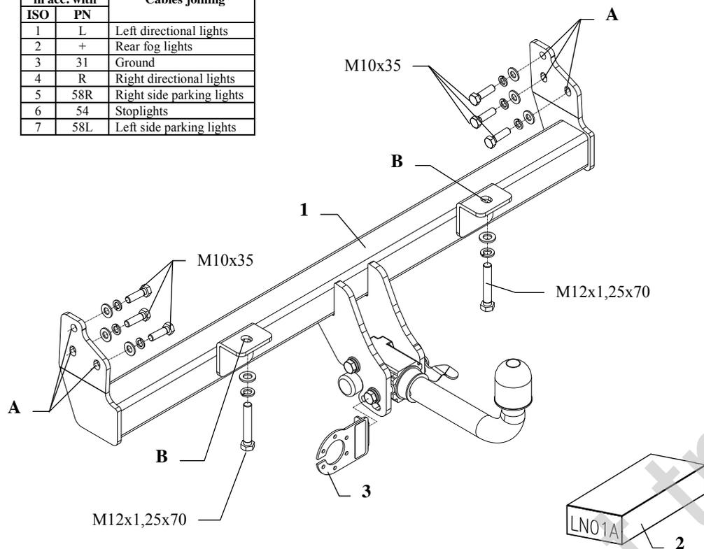
This towbar is designed to assembly in following car: **LAND ROVER FREELANDER, (LN)**, produced since 03.1998 till 09.2006, catalogue no. **LN01A** and is prepared to tow trailers max total weight **2000 kg** and max vertical load **140 kg**.
