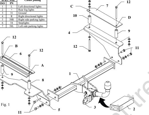
This towing hitch is designed to assembly in following cars: CHEVROLET AVEO, 4 doors, produced since 03.2006 till 07.2011, catalogue no. X21A and is prepared to tow trailers max total weight 1200 kg and max vertical mass 75 kg.
